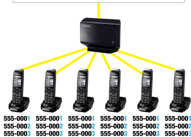
6 Station: 3 Line "Key" System
